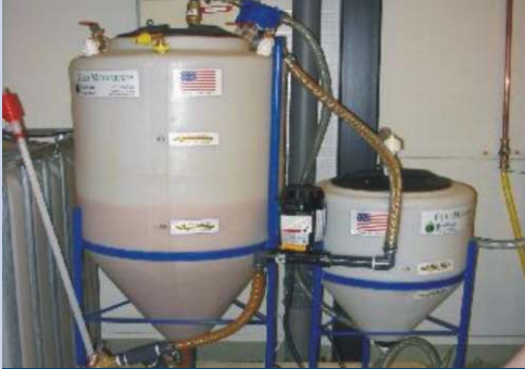
Small Scale Biodiesel Plant
